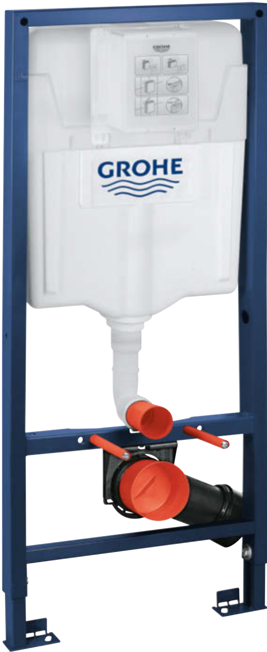
38 528 001 Rapid SL for WC with flushing cistern 3 – 6 l dual flush/start & stop/single flush connection from left/right/rear 1.13 m installation height
