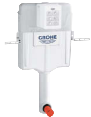
38 987 000 GD2 WC Flushing Cistern 6l/3l Dual Flush water supply from top/back includes inlet pipe & connector without wall plate/actuation for mounting of small flush plates please order inspection shaft 40 911 000 (sold separately)
